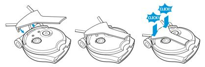
► Connect the induction loop 28 to the socket 5 of the receiver.
